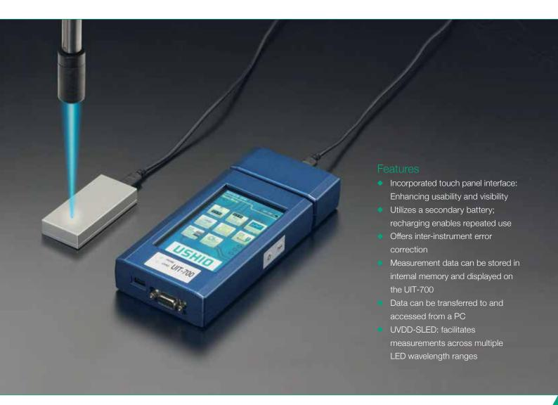
The UIT-700 is an advanced UV meter renowned for its exceptional functionality, capable of measuring a broad range from  $0.1 \, \mu \text{W/cm}^2$  to  $25 \, \text{W/cm}^2$ , within a single unit.
