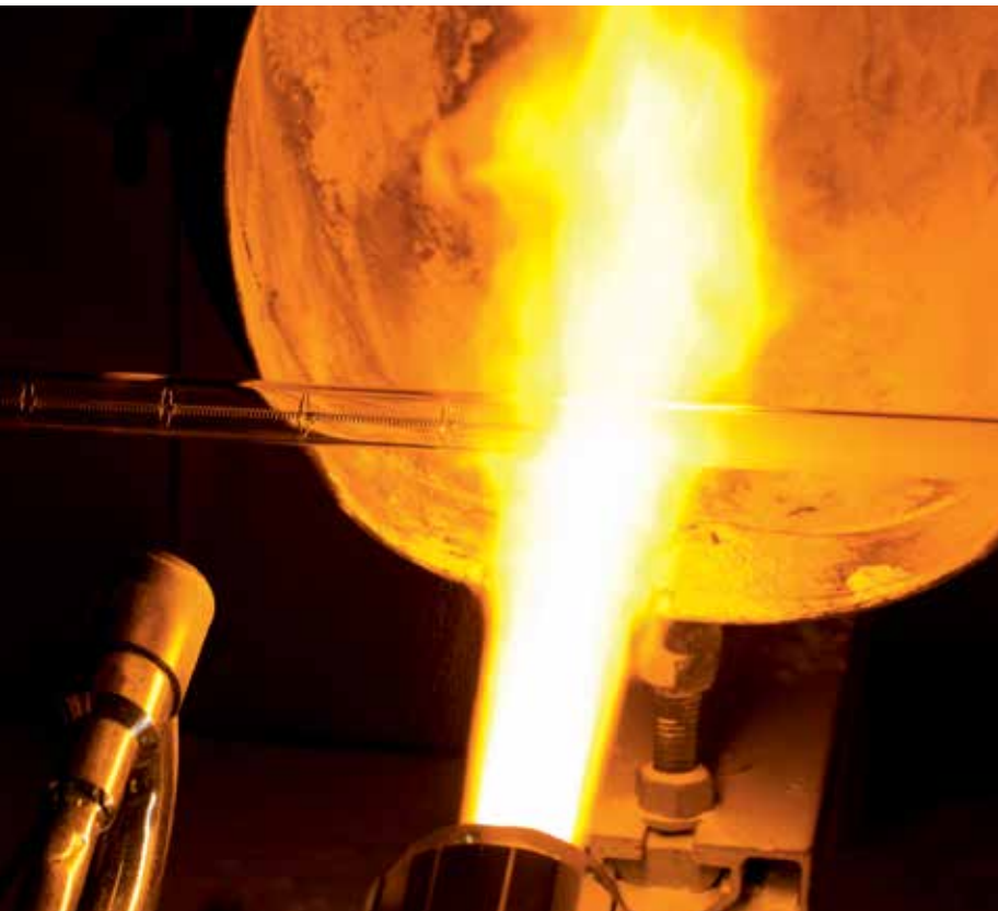
Flame spraying the quartz tube during lamp production
