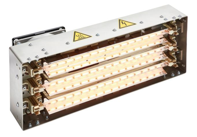
Ushio's engineering division developed a series of infrared modules and auxiliary components that serve as basic building blocks for many typical IR heating processes. The Ushio IRtenser heating modules emit of short-wavelength infrared radiation in the 0.8–1.5 µm range, with a power density of 200 kW/m<sup>2</sup>. All IRtenser modules feature an integrated air cooling system, EmitFit quick-release lamp mechanism, and are delivered ready for immediate use.
